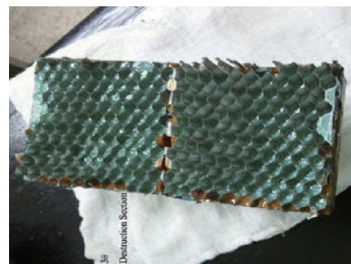
图8 FM-73M平拉试验后图片 Fig.8 Image after FM-73M Ping-pull test
